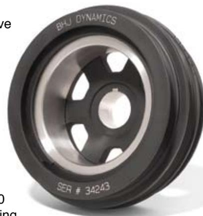
Both S.F.I. and E-Performance Harmonic Dampers are custom designed to meet each specific application and all critical O.E.M. mounting dimensions are duplicated for accurate alignment of accessory drives. All Harmonic Dampers feature a T.D.C. mark and when necessary, are degreed from 0 to 50 degrees in 2-degree increments for accurate ignition timing. 90-degree marks are also included for easy valve adjustment.
