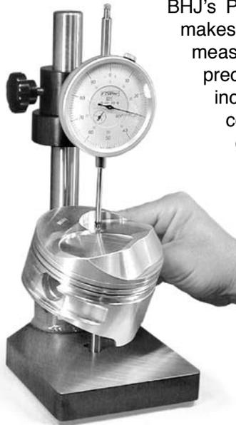
The Dial Indicator is mounted in a Sliding Collar and is supported by a Locking Collar that has a radial stop, which allows precise alignment of the Anvil Tip with the Indicator Tip. Set-up and operation procedures are simple and can be performed by any qualified machinist.
