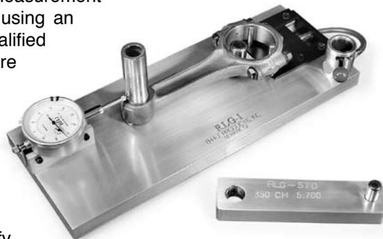
The Fixture accommodates automotive connecting rods with an approximate center-to-center distance of 5" to 8" and a big-end I.D. range of 2.100" to 2.750". A precision Dial Indicator and one application-specific Length Standard are included in the Kit (specify application when ordering). Additional Length Standards are also available for most connecting rods.
