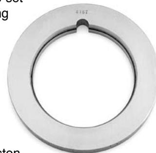
Each Gauge is accurately machined to size with an internal Step to square the piston ring and features a Relief that is added for clearance of a feeler gauge when taking gap measurements. The bore size is machined in the top surface of each Gauge for easy identification.
