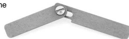
The angle relationships are quickly checked by first pressing the Comparator to the valve head to set the angle (Illustration #1), then placing it on the piston to check the piston relief angle (Illustration #2).
