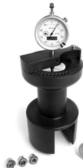
BHJ's Valve Margin Comparator enables quick and easy comparison of valve margin thickness. Detecting margin variations between valves is critical to matching their flow characteristics, as well as assuring equal combustion chamber volumes. Matching the valves before head assembly reduces the possibility of disassembling one or more chambers after cc'ing the head to re-machine the valves or seats.
