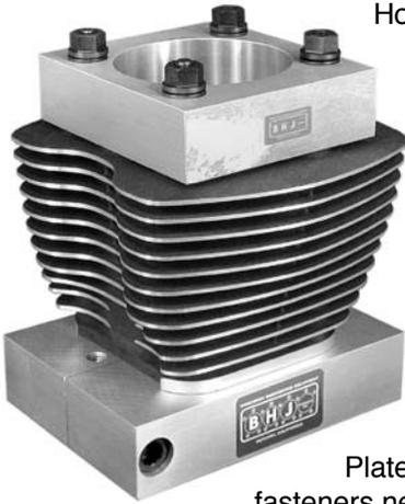
Honing Plate Kits are available for the Harley Davidson Shovel Head, Evolution and Twin-Cam engines. Kits are supplied with a Base Plate, which features side clamping of the spigot area on the Jug to address the recurring problem of spigot deflection during honing. This is especially prevalent in large-bore applications and will eliminate additional clearance that would be necessary to achieve correct piston to cylinder wall clearance.
