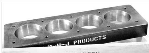
When a cylinder head is installed on the block, substantial valve seat distortion can be measured from the stresses induced upon the head, thus compromising the valve seal. Having the ability to grind or cut the valve seats in this distorted condition is advantageous to proper valve-to-seat sealing.
