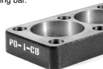
In order to maintain the closest possible block distortion, it is necessary to use the same type of cylinder head gasket that will be used during final engine assembly when conducting the honing operation using the CB Model Honing Plate.
