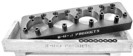
The R Model Honing Plate is the established standard for duplicating cylinder bore distortion and is a must for any high performance engine application. Used by top machine shops, racing teams and racers alike, the R Model is acknowledged to be the finest, most accurate honing plate on the market today.
