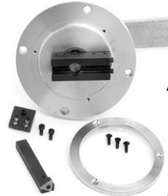
Groove diameter is precisely set using a special Dial Indicator, which is included with the Cutter. Accuracy of the groove diameter is within .002" and groove depth is easily adjusted with the built-in micro stops, with accuracy within .001". Diameters range from 2.400" to over 5.125", based on application.
