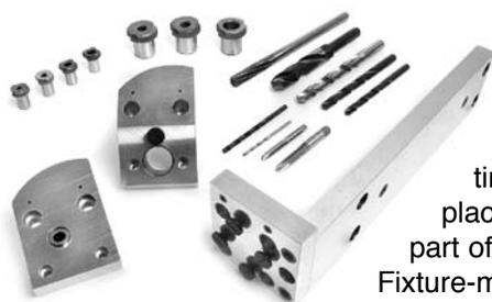
The Kit is installed via a Registration Plate, which precisely aligns from the timing cover locating dowels using hardened bushings, and bolts securely into place. Three Fixture Blocks are attached to the unfinished boss to execute each part of the three-stage process. The Kit includes all the necessary Fixture Blocks, Fixture-mounting Hardware, Drill Bushing Guides, Drills, Taps and Reamers to do a clean, precise job every time.
