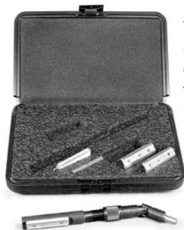
BHJ's Lifter Bore Honing Kit contains everything needed to make fast work of final-sizing lifter bores. The rigid style Hone utilizes a friction Thimble and feed Wedge for increasing diameter and is operated with a 1/2" drill motor. With a diameter range from .843" through .937", this one Kit will accommodate Chevrolet, Ford, Mopar and Jesel lifter bores.
