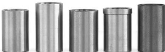
BHJ's Lifter Bore Sleeves are available in both SAE 660 Bronze and A-48 Cast Iron in a variety of sizes to suit standard Chevrolet, Ford and Chrysler I.D. applications. Standard Lifter Bore Sleeve (Lifter Bushing) sizes are nominal 1" O.D., by 1.500" long and are of a standard "Barrel Bushing" design.
