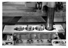
The Bor-Tru Kit consists of one Deck Plate, which is engine family specific, one pair of universal Alignment Bars, which fit any V-8 or V-6 engine application, one Set-Up Spacer, plus all fasteners necessary for assembly. Optional Counterboring of the Plate Bolt Holes is available for use with a deck-mounted or portable boring bar, or any type of boring equipment that must contact the deck surface of the block while boring.
