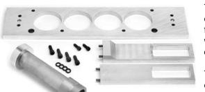
The Bor-Tru is a specially designed Blueprinting Fixture for establishing correct cylinder bore and dowel locations on semi-finished cylinder blocks, as well as any stock factory block, when a sufficient overbore will allow correction of out-of-position cylinders.
