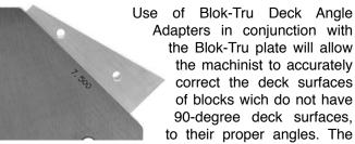
adapters magnetically adhere to the index surface of the Blok-Tru plate, allowing the block to be indicated in flat or parallel from the top surface of the adapter.
