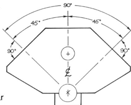
When the Blok-Tru is set-up and used in the prescribed manner, all angular dimensions shown in the illustration can be held within five minutes of one degree.
