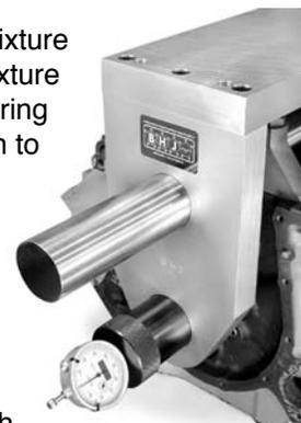
Step-Up kits may be purchased to upgrade to different engine families and are supplied with one pair of End Plates. Also available is the Small Block Chevy Distributor Alignment Fixture, which indexes the cam tunnel honing location to the blueprint-correct distributor gear "sweet spot".
