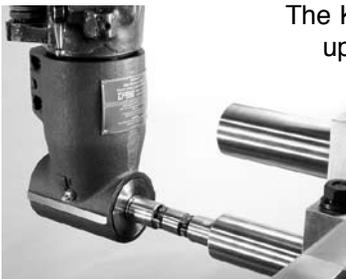
The Kit contents include all of the necessary Positioning and Clamping Hardware for set-up, one Boring Bar (for cam or mains), set-up Dial Indicators and a 90-degree Drive Head, which mounts to an existing vertical mill. An instructional DVD is included with each initial kit and is also available separately by calling BHJ. Also available is the Small Block Chevy Distributor Alignment Fixture, which indexes the cam tunnel boring location to the blueprint-correct distributor gear "sweet spot".
